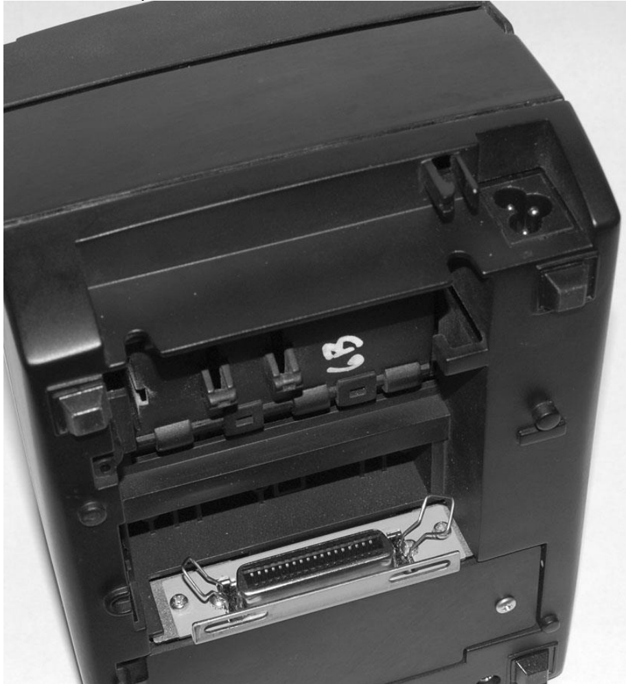
Figure 7. Communication PCB Location and Connector Info.
